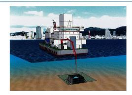
Marine-environment compatible distributer with a 30-meter boom enables direct placement as well as high-quality underwater placement.
